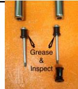
**STEP 6** Use a liberal amount of grease on the spring and reinstall spring and preload cap back into fork. Torque to 5-6Nm.
