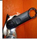
**STEP 3** Pull up carefully not damage the spring retainer at the end of the spring preload knob. Put aside and move on to pulling off bottom out spacer and rubber bumper. Once those parts are removed turn the CSA (Crown, Steer Assembly) over to let the compression rod come out of the top of the crown to inspect
